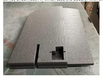
Once dry sand the leading edge to profile, the wing cut out in the fuselage sides will show what you are aiming for. There is no need to sand the TE and it is beneficial to leave it square!.
