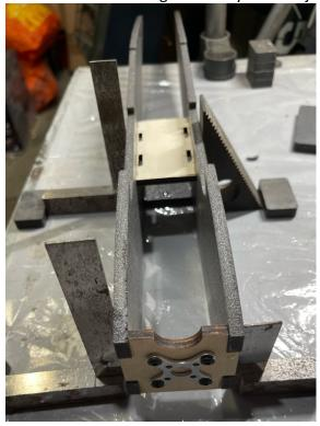
When all the formers / spacers, trays are dry then fit the fuselage top, bending the rear of the fuselage sides in to match the curve. To make threading cables easier fit the rear fuselage mounted elevator servo, I use hot glue to hold it in place.
