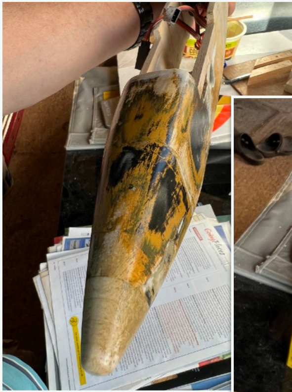
Sealed with 2 layers of Eze-Kote, the nose is sprayed with car body primer/filler.
