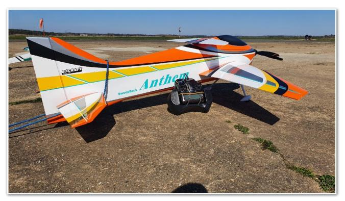
After assembling the model and checking everything over yet again, I did the obligatory range check and got a club mate to move the model through 4 quadrants to check the radio reception while doing the range check. All checked out as did the Failsafe check.
