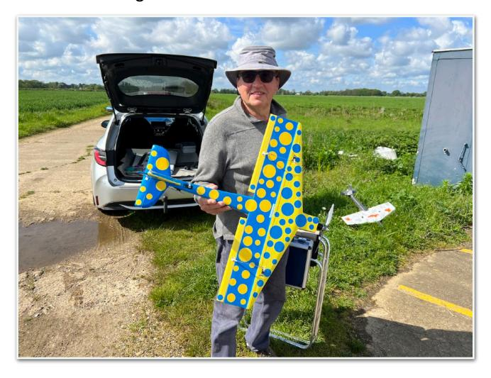
He has retained the style of the original KFm-2 aerofoils built, keeping the 'steps' parallel with the rear of the wing.
