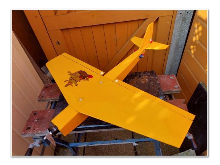
Standard motor, 9X6 Prop & 1400 mah battery (140g) yields a flying weight of 550g.
