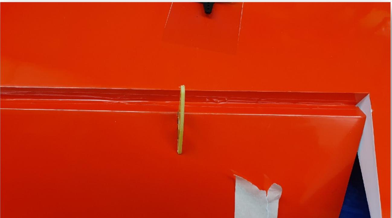
I did the same for the elevator hinge gaps. However, the rudder has multiple colours and so I will use transparent tape to seal the rudder hinge gap.
