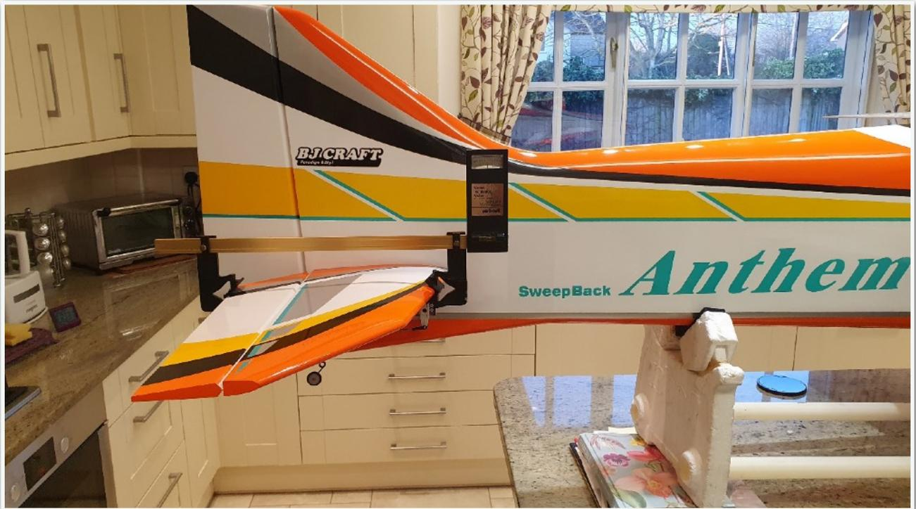
In order to achieve an accurate reading, you must have the radio system on so that the elevator and aileron servos can hold neutral with the weight of the Robart incidence adjuster resting on them. I fine tune thickness of the packing by only using part of a magazine as you can see in the photo below!
