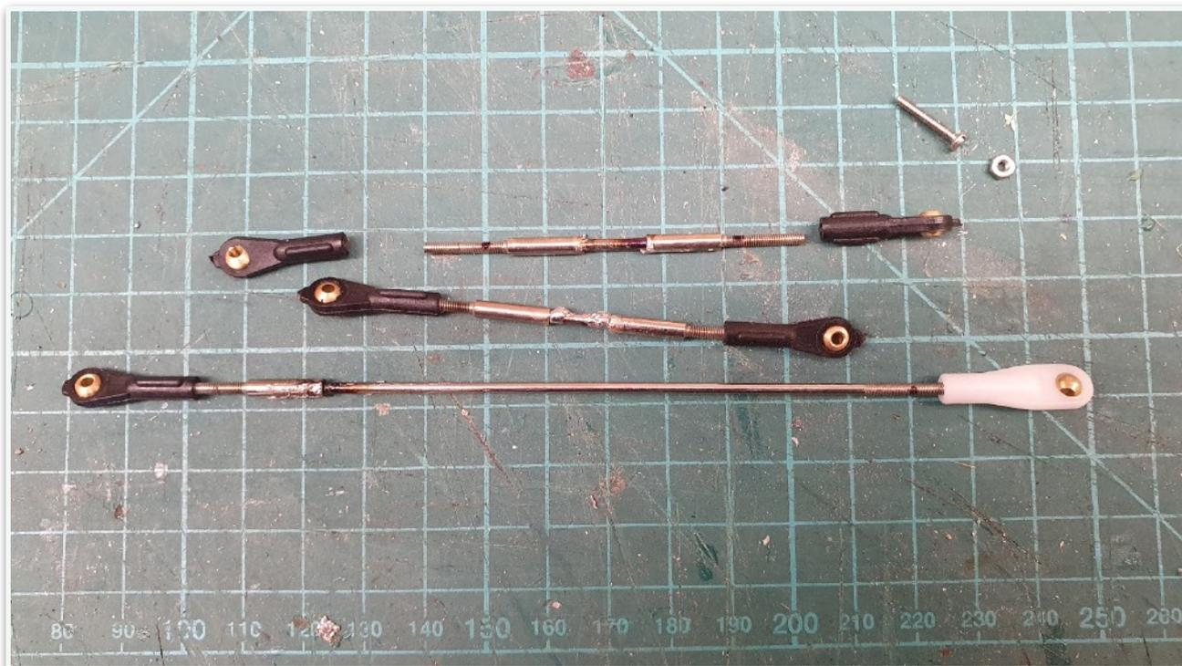
After that, it was just a matter of getting their length right so that the ailerons were flush with the wing and the rudder central when the rod was installed. It's important to note that you should zero any sub trim you may have on the servo and then fit the servo arm so that it is parallel with the hinge line of the control surface.
