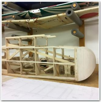
I used a one piece 1/8 ply dihedral brace on the centre section rather than wing tubes to keep the weight down: this made the joining of the two halves of the centre section a complicated procedure, as the brace is first araldited to one half and when set the the second half is slid on and glued on place.
