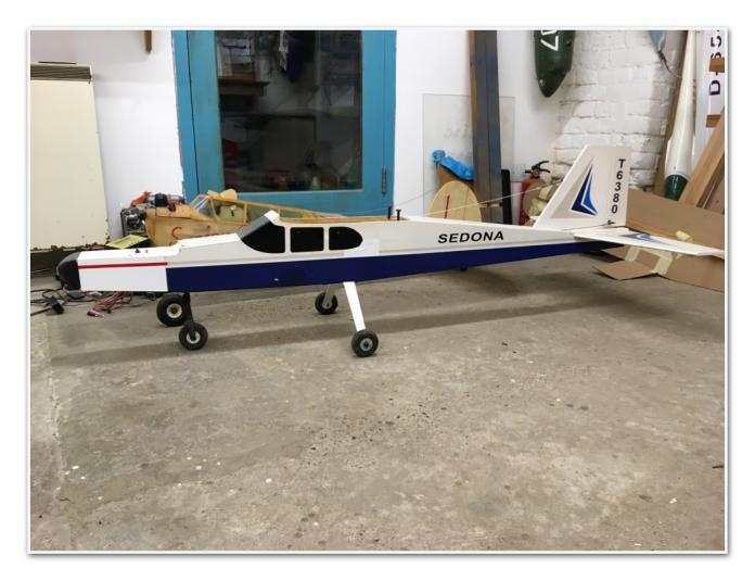
Wing, tail feathers and fuselage finished, next step is to put it all together and add weight where the engines will go to see how far forward of the leading edge they need to go to achieve balance so I don't need to add any weight.
