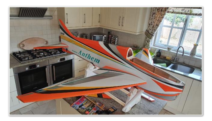
As it happened, the fixed location of the wing indicated that B J Craft had managed to get their jigs spot on as the wing incidence came out at 0.7 deg! While I was de-rigging the aircraft, I took the opportunity of checking the wing sweep and the kitchen floor tile pattern provided the ideal way to do so! It's about 18-19 deg sweep back.
