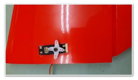
As you can see, the servo is a very snug fit and the provided servo tray was designed for a thinner servo. So having measured how deep I wanted the servo to go, I then eased the ply servo plate into position, sanded to give a tight fit, then secured it with cyano and cut off the ply joining the ends of the tray. That allowed the servo to be positioned, holes to be drilled and the servo bolted into place.
