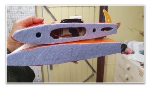
As you can see from the photo, I drew 2 lines to show the position of the carbon tube marking its depth of engagement as well. Careful application of the drill provided the connecting hole in the carbon tube and, phew, both screws worked as required!
