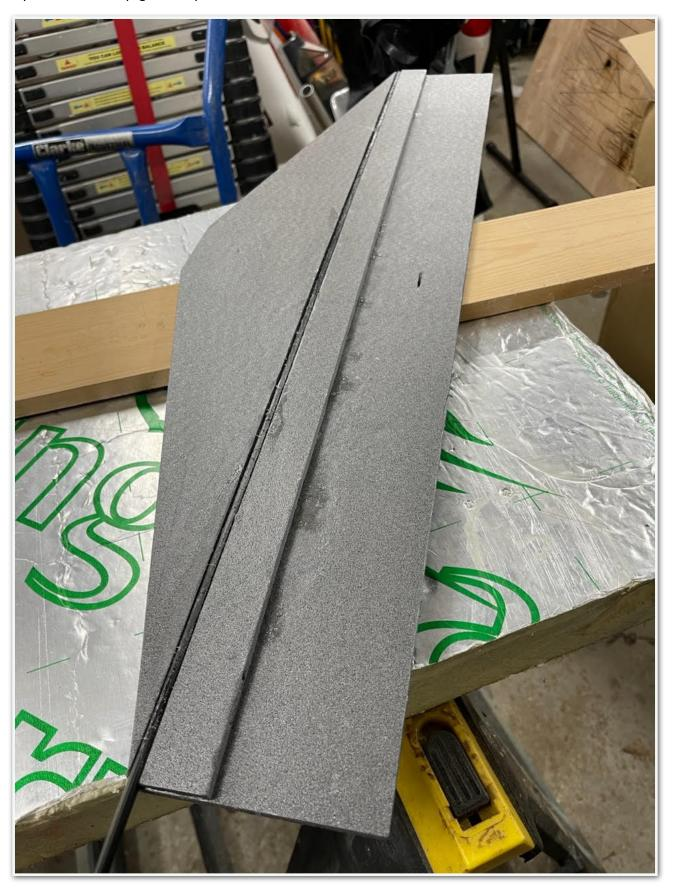
It's loosely based on the KFm-2 aerofoil which has the step at 50% chord. Not sure how that relates to a swept LE wing like the Hanky Planky so will be interesting to see how it performs.
