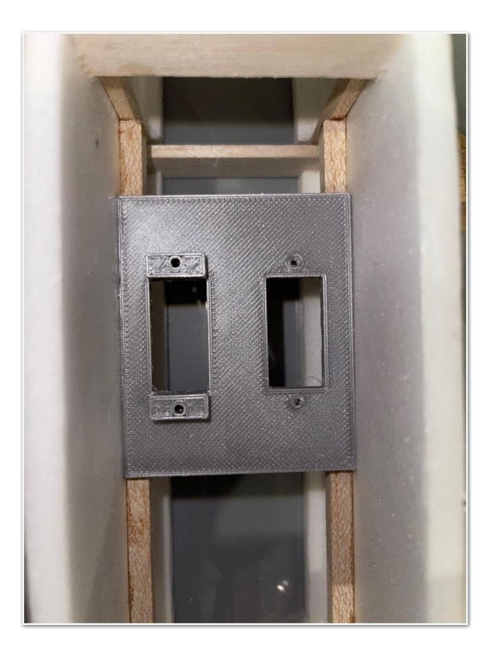
The engine former was marked and drilled and then glued in position with some balsa strengtheners behind.
