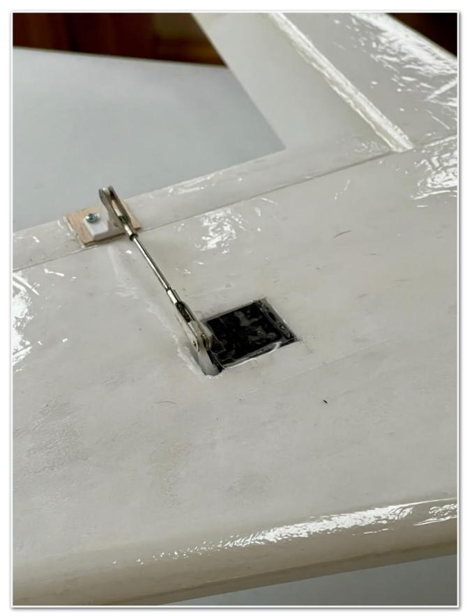
Finally the under fuselage battery access hatch was hinged using reinforced tape and a latch made from an old servo horn.
