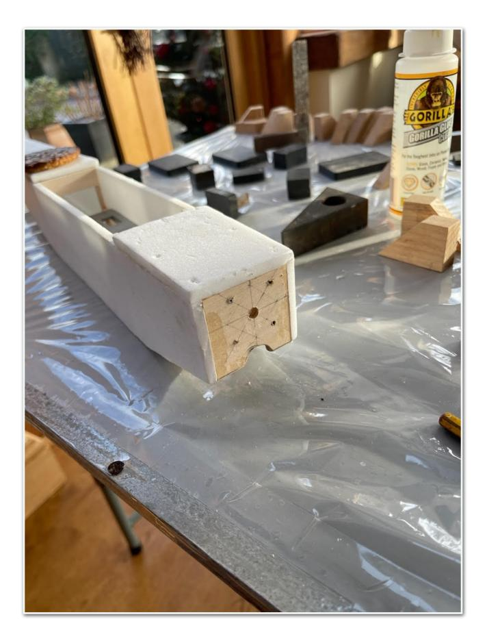
Underside nose and belly sheeting was then added to complete the fuselage 'box'.
