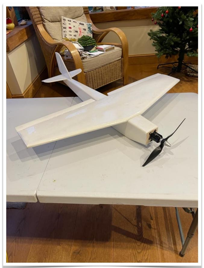
I originally planned for the tail servos to be fitted on the 3D printed servo tray in the fuselage. When I came to check the C of G it was apparent that the model was very nose heavy so I decided to fit them into the tail of the fuselage rather than having to add weight.
