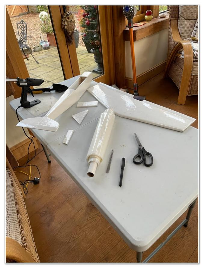
Next I stuck the tailplane to the fuselage followed by the fin which had a couple of cocktail sticks stuck in it and through the tailplane for additional strength. All hinges were formed by the 'overlapping covering' method with the exception of the rudder which uses mylar hinges. I couldn't resist putting it together for the next shot!
