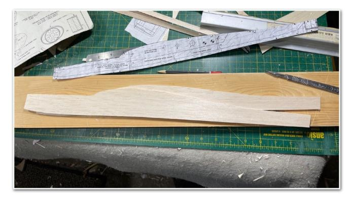
Which had thin ply doublers glued on together with triangular balsa bottom fillets.
