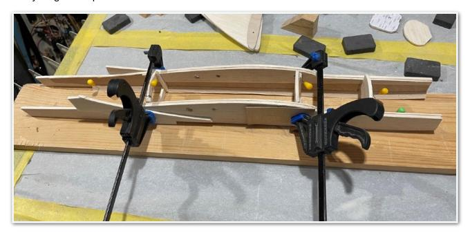
The build instructions and plans show a ply and balsa motor mount / rear former made by bending strips of ply around a former.
