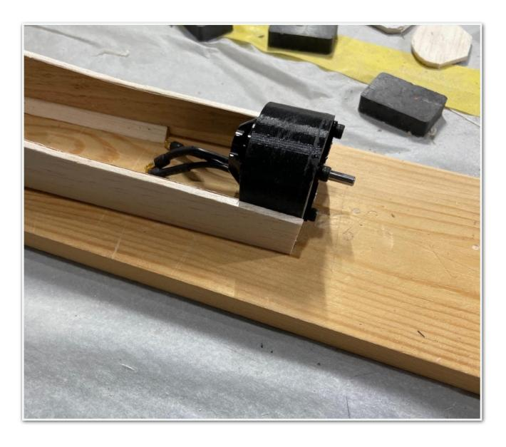
The front former was added as were the ply canopy side rails but they were held in place with double sided tape, the idea is the the canopy planking is stuck in place onto the ply side rails then it is cut out once dry
