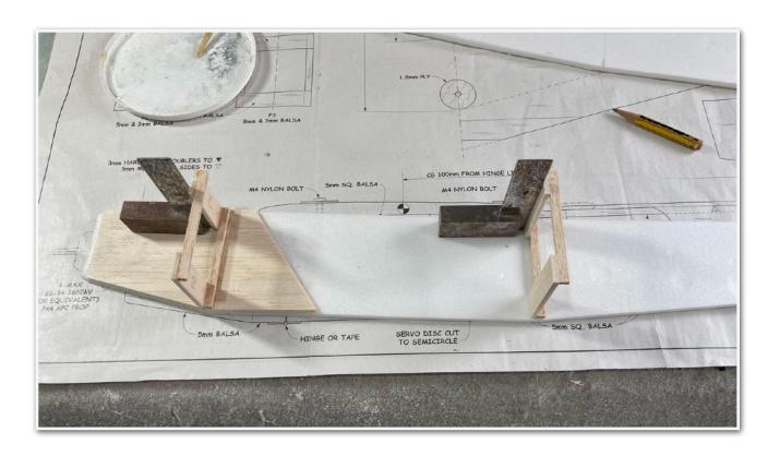
Note the additional strips of foam along the edges of the fuselage sides, this gives a greater gluing area and also means that the edges of sides cap be rounded.
