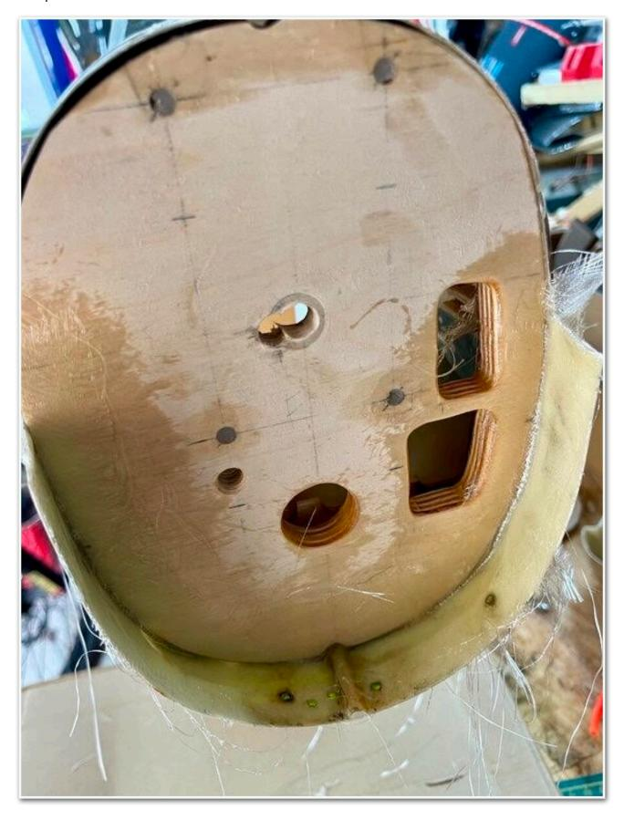
As with most IC, the height of the fuel tank can be critical but it is especially so with Laser engines and as their carbs sit quite high (low when inverted) the tank needs to go quite a bit lower than 'normal'. In order to achieve this a tank recess had to be cut in the top of the wing and the opening lined and glassed to maintain wing strength.
