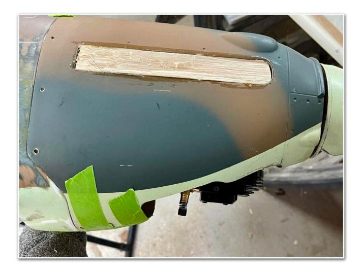
(Balsa on the exhaust port is where I cut off the previously fitted (hideous) exhausts, which will be replaced with 3D printed ones.)
