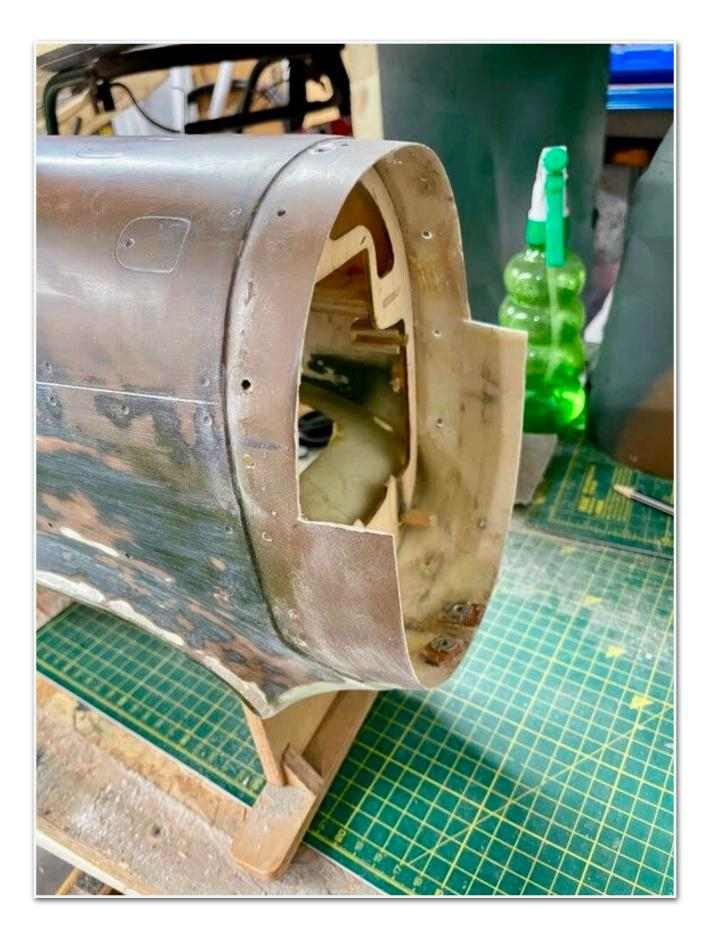
The new bulkhead (12mm ply) will sit in front of the former you can see in the last photo by 13mm so to give more strength to the top half where I've cut the fuse back I cut a backing former
