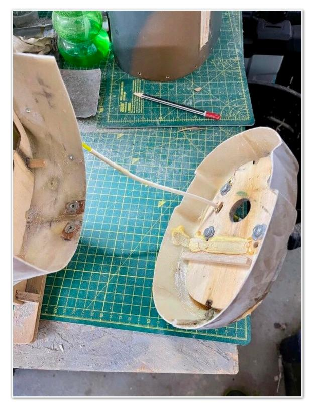
I then cut back the top half of the fuse so that the new bulkhead can slide down from the top:
