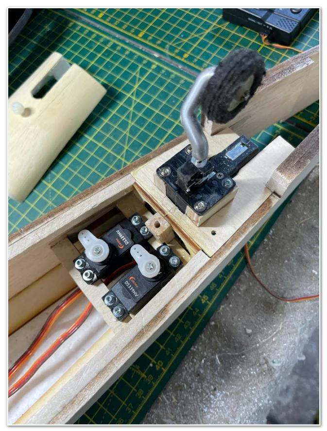
But what with the rear mounted servos and the retract unit I then needed some form of access hatch for them. To achieve this I cut out a section of the veneered foam under fuselage cover and mounted this with a nylon bolt.
