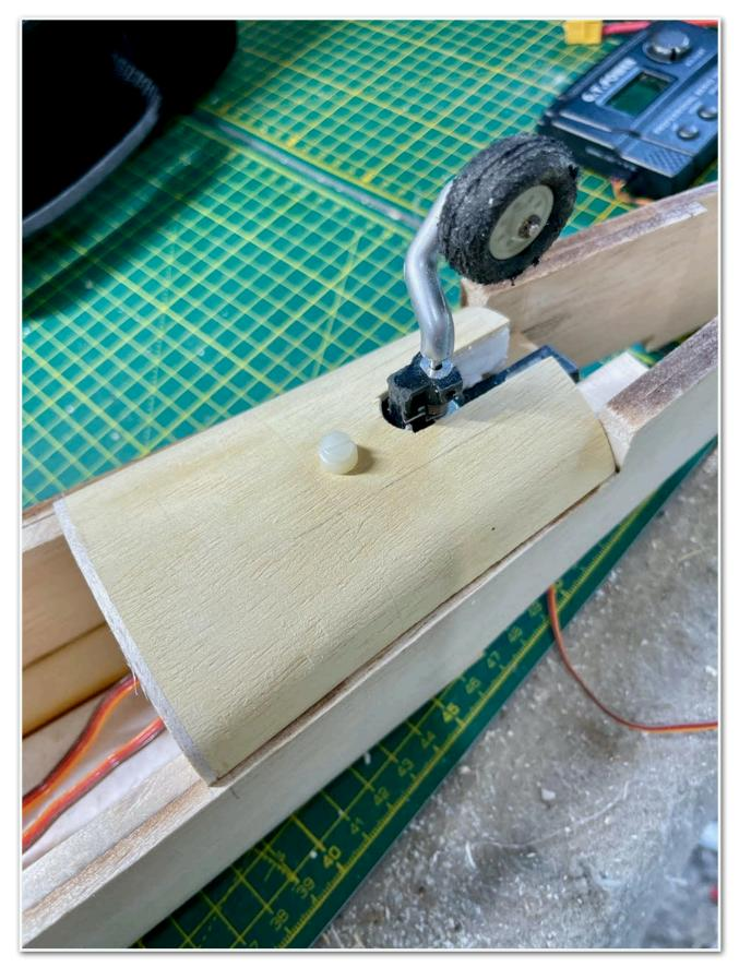
I could now glue the front section of the under fuselage covering.
