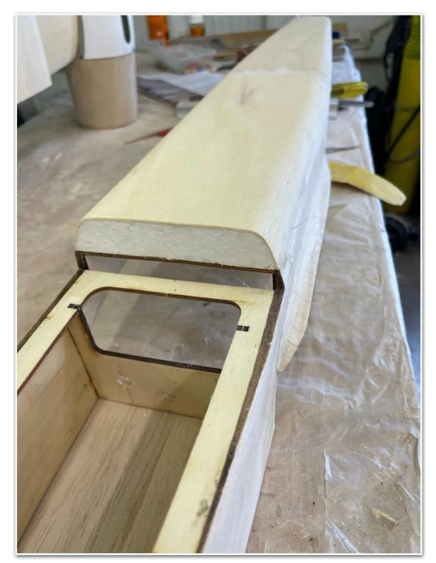
Block balsa for under the nose (note holes drilled for wing mounting dowels).
