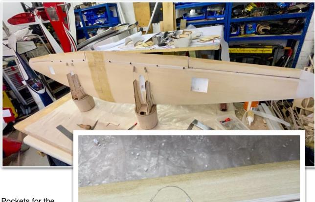
Pockets for the flap mini servos were cut out and the servos fitted using 3D printed servo mounting plates.
