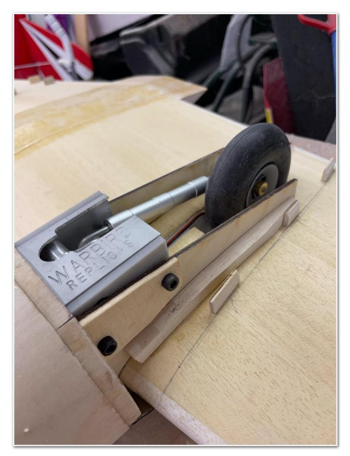
A trial fit of the plastic nacelle underside covers shows that very little of the wheels will protrude when retracted.
