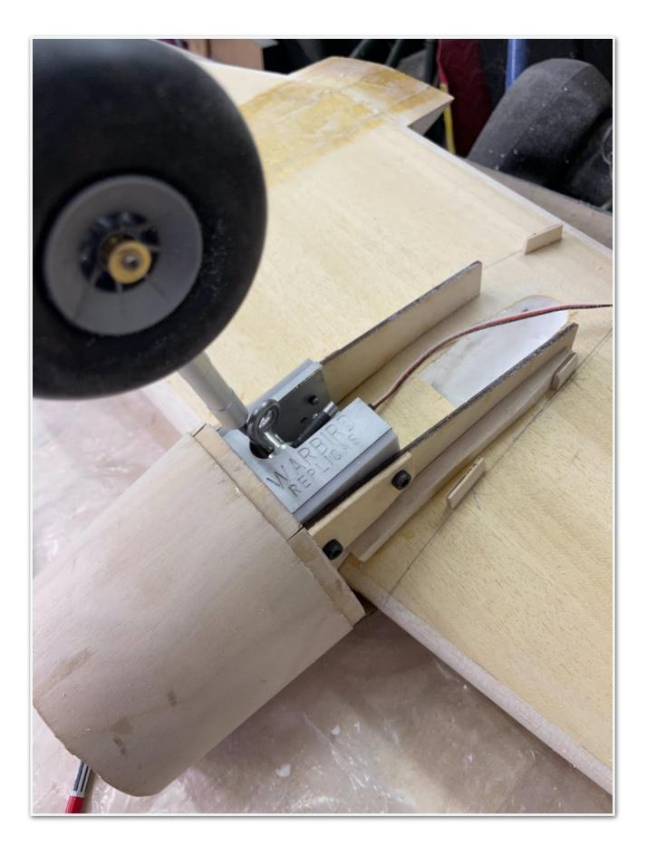
Recesses cut into the wing allow the wheels to retract quite deep.
