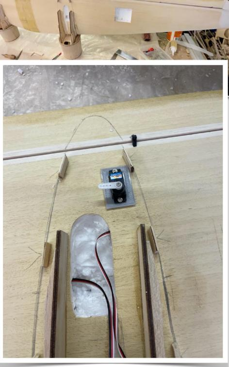
Similarly, the aileron servos were fitted using 3D printed servo mounting assemblies fitted to ply servo boxes.
