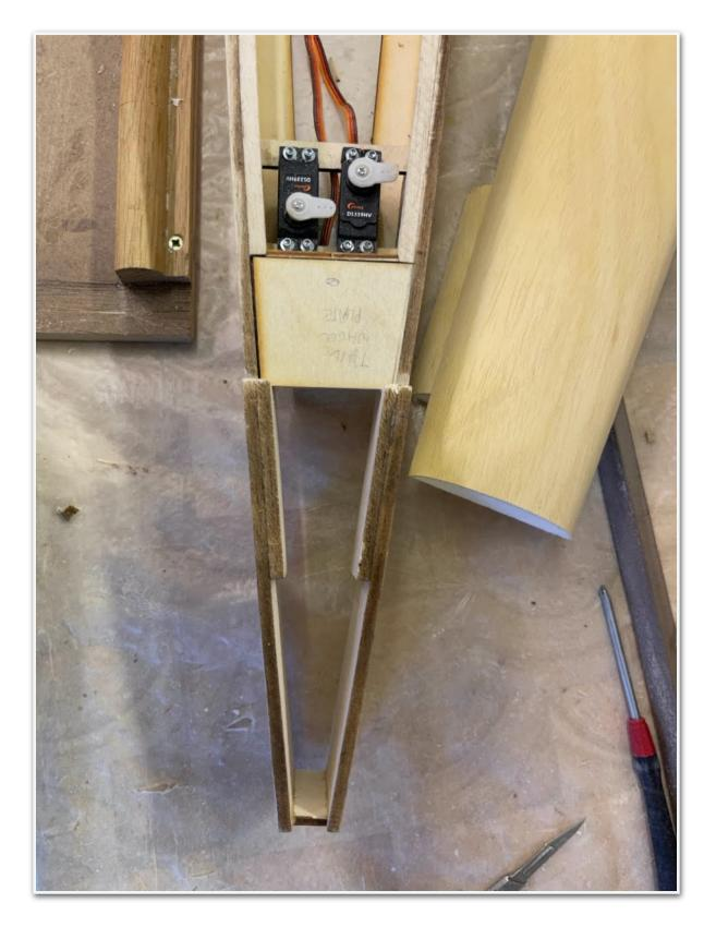
And at this stage I was still going to mount a fixed tailwheel. However, as I had a weight advantage I thought 'what the hell' and went about modifying an older tail retract that I had in my spares drawer and attached a mounting plate for it.
