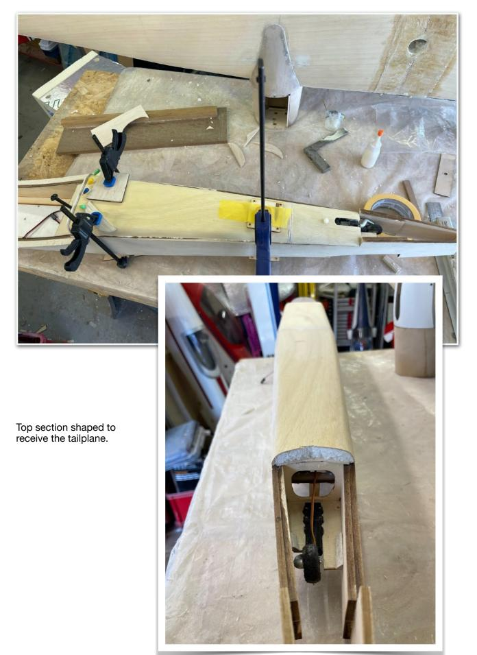
The underside showing the access to the servos and retract.
