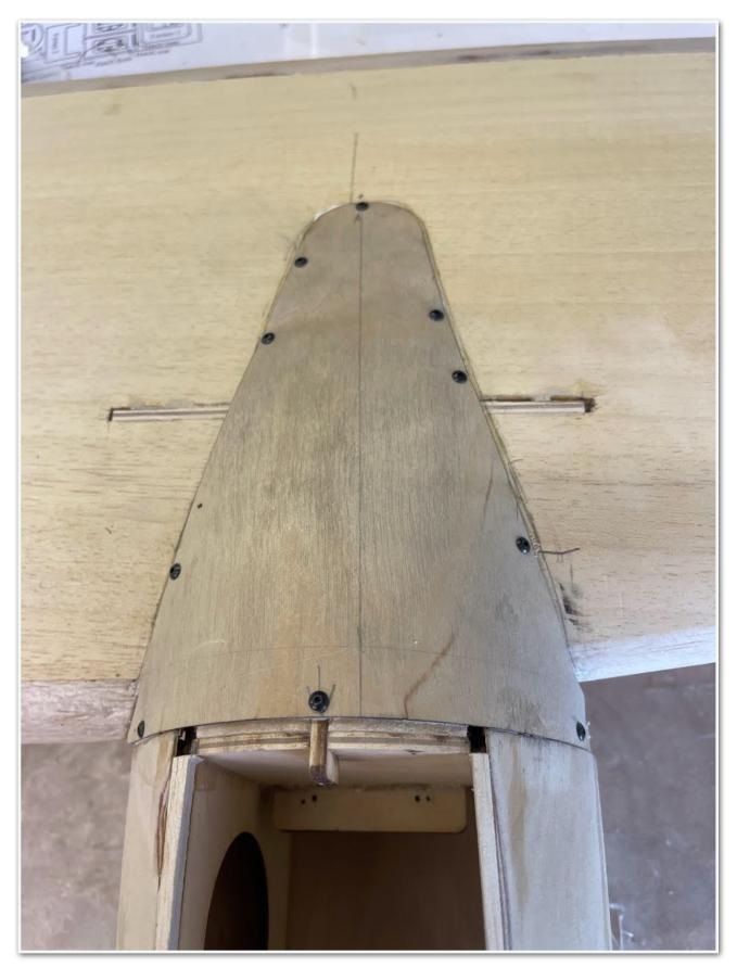
Next up the fitting of the retract units which have been specially manufactured by Warbirds Replicas to suit models like this where the U/C folds back into the nacelles. Due to their construction the fixings are through the sides so I fitted some ply strengtheners / load spreaders to the sides of the nacelle frames.
