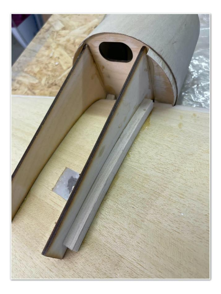
After which i was able to attach the thin ply nacelle covering using small screws to hold it in place whilst the glue dried.
