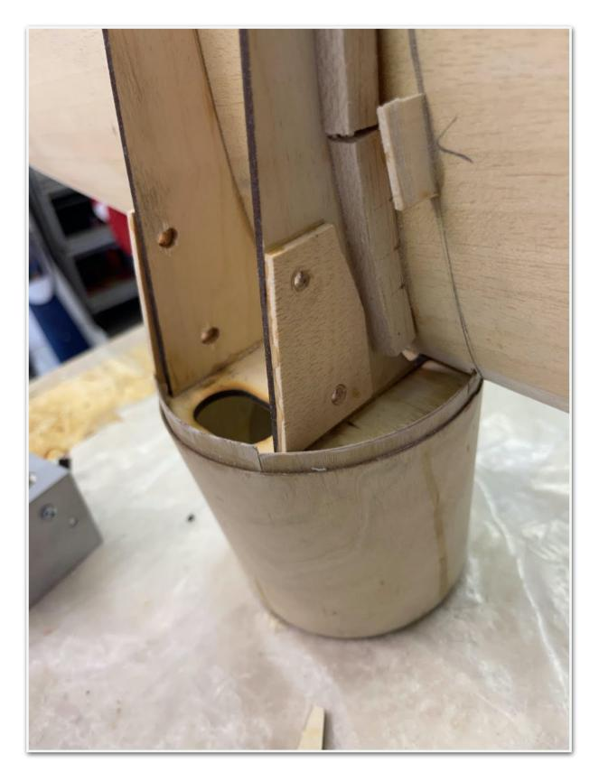
And packing pieces to take up the space between them and the retract units in which I had tapped holes to take the fixing bolts.
