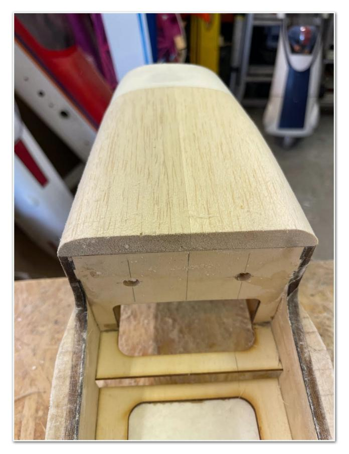
Rear half of plastic nose fitted to ply former and glued to fuselage.
