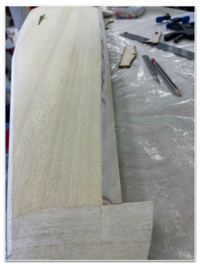
I also cut out the aileron servo pockets again using the soldering iron gun / hot wire cutter.
