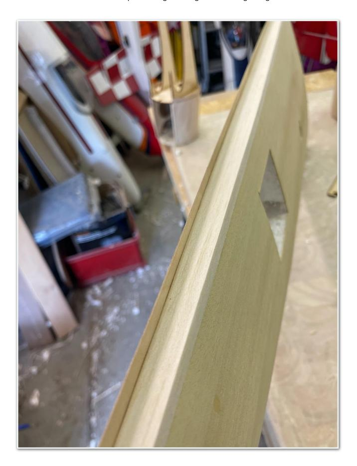
The 2 halves of the wing were then glued together (Gorilla Glue Brown).
