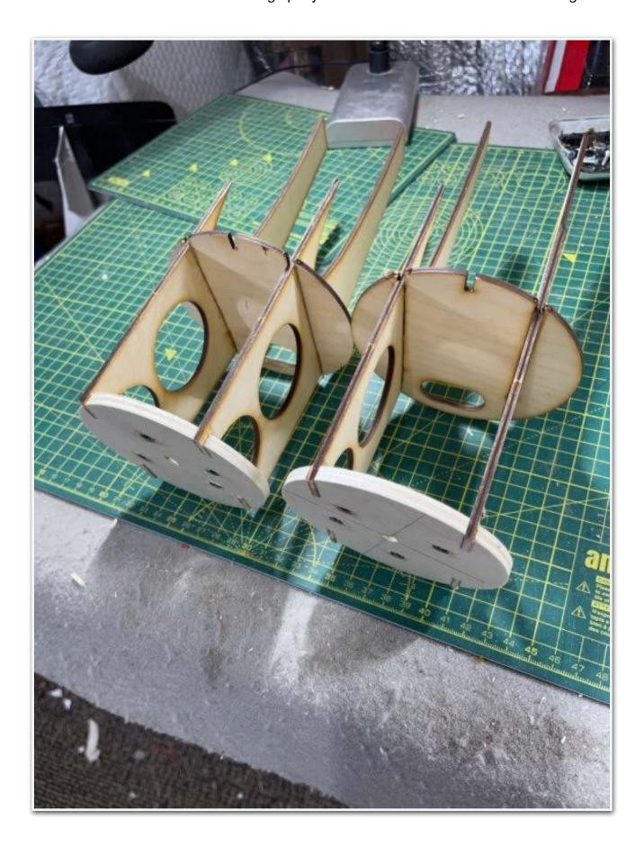
Motor mount loosely attached. Note that I cut out a section of the top of the motor mount to allow the motor to fit tight against the firewall (thanks for the tip Richard).
