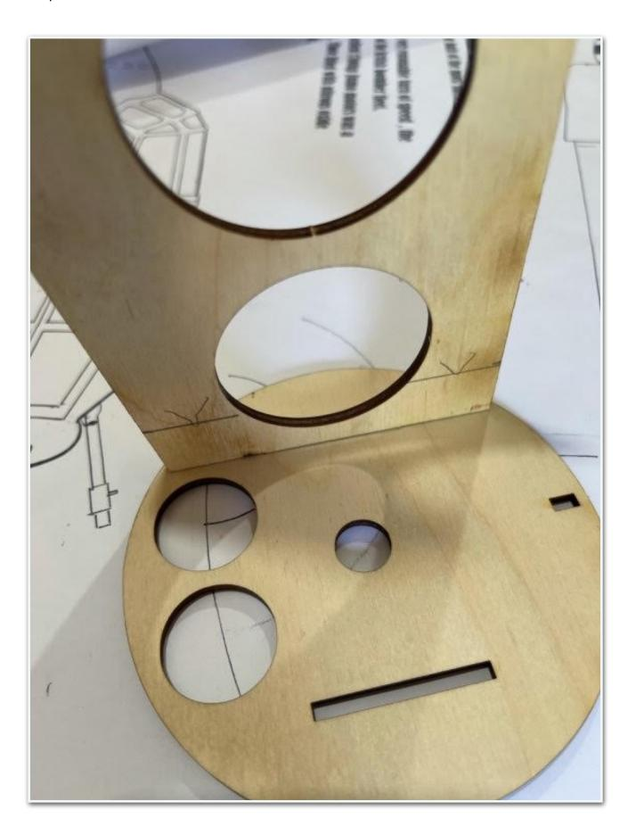
Whilst I know that the firewalls (designed for leccy) will be fine I've decided to make new ones from 6mm ply (the circle in the middle was drawn before I realised that there was a saw cut! - I hate waste).
