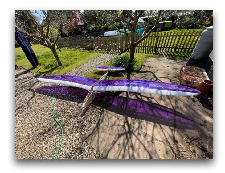
I had a big problem covering the rudder, the transparent HK film really does shrink, a lot more than the solid colour stuff, and it twisted the rudder like a crisp. Second attempt, at a lower temperature, wasn't much better so I added some diagonal braces to the structure then applied the film at an even lower temperature and this time it was OK.
