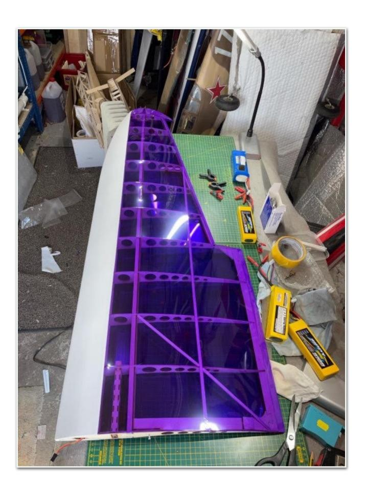
Time to sort out the wing to fuse fixings. The design is for 2 hooked screws fixed to the root ribs and then once the inner wing panels have been slid onto the joining plates a rubber band is used to hold the wings together. I didn't want to do that, I wanted to have nylon fixing bolts instead.
