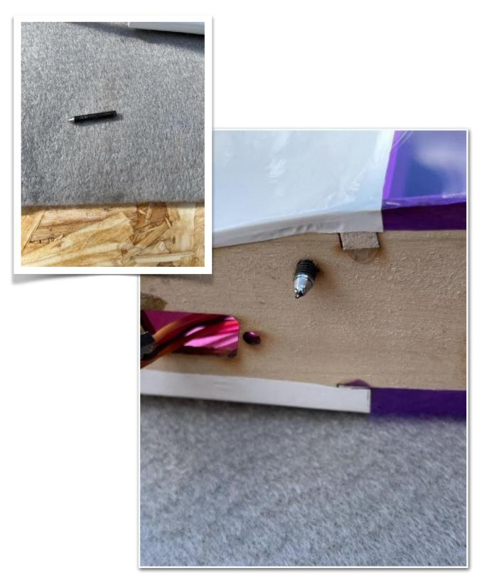
Then I pushed the inner wing panel into the fuse so the the pin formed a slight indent showing where to drill the hole for the fixing bolt.
