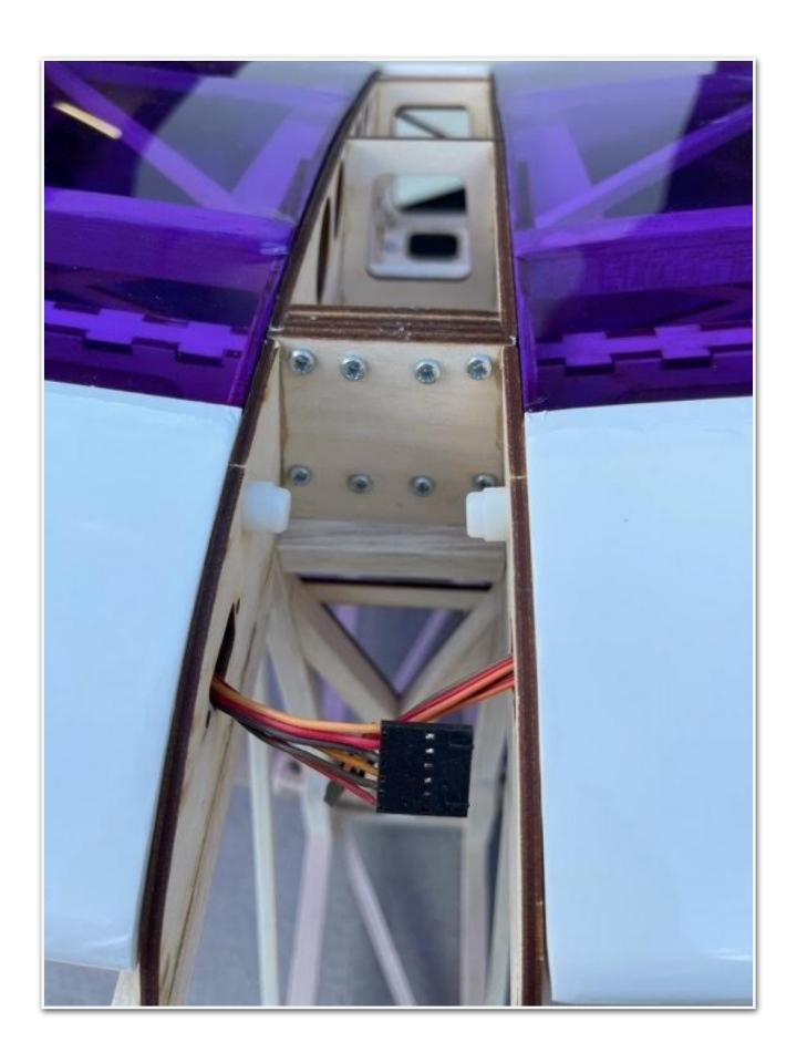
I wanted to check the C of G so put the wings together and fitted them to the fuse. With a 3700Mah 4s up front it balanced ok.
