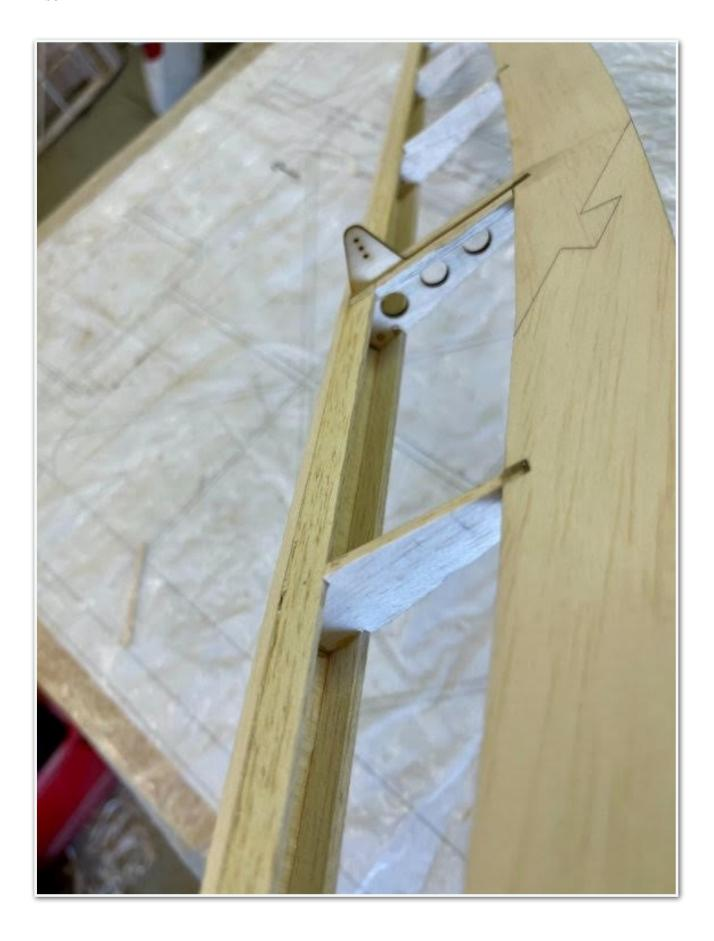
Which resulted in a straight LE, the horse has been fed! (The patchy look on the TE is where I've still got to go over it with the iron and cloth).
