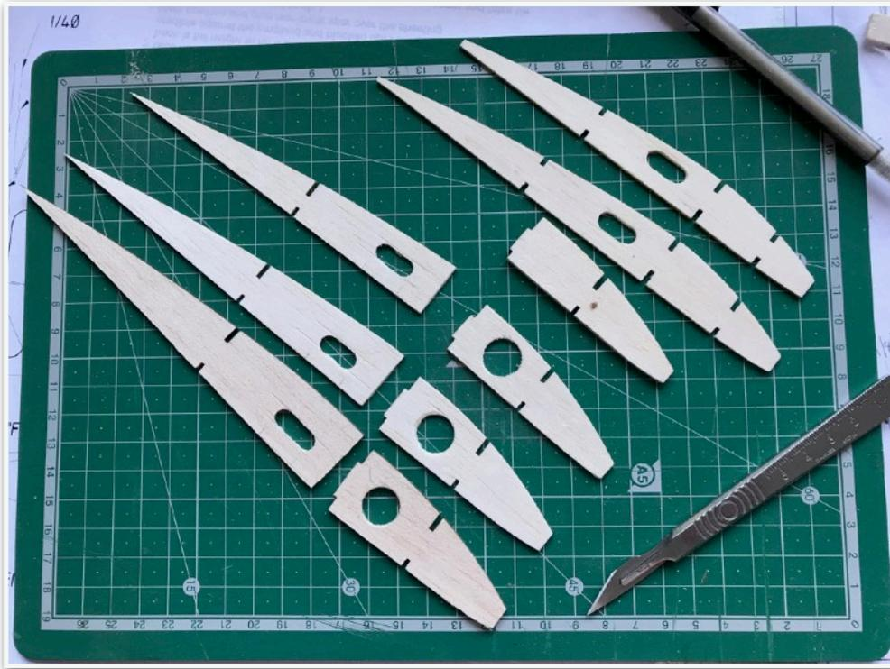
It had the advantage that I prepared the ribs for wiring before attaching them to the lower sheeting.
