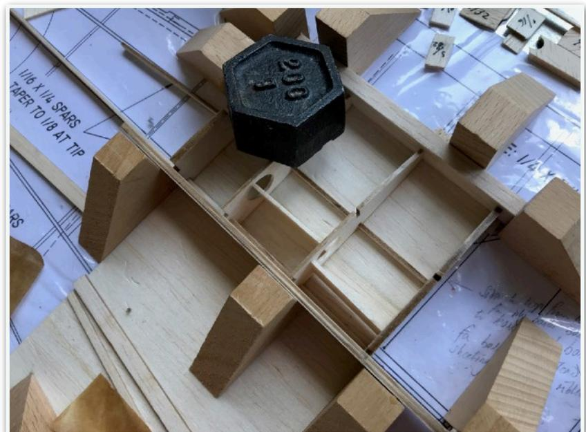
I added rib 1, then used it and loose fitted ribs 2 and 3 to get the spars in place, both forward and aft of the temporarily fitted brace.
