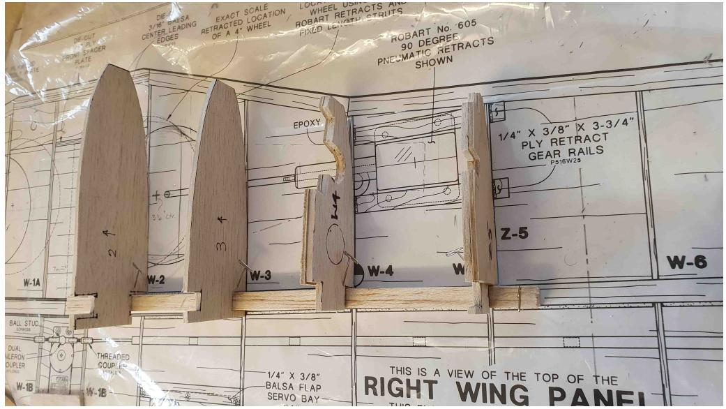
So this photo shows my mock up in construction. I've decided not to cover the top and bottom with 1/16 inch skin so the completed structure, still drying out, is below.
