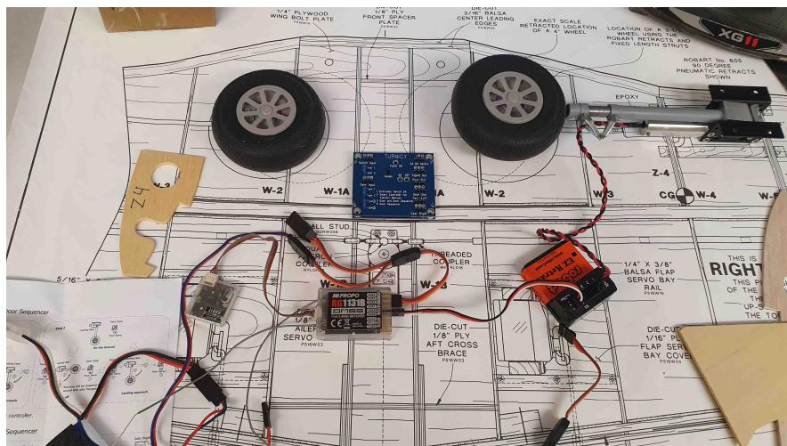
lead coming out of the Gear plug on the Rx and connecting the HK sequencer to one lead and connecting the inner door servos to that controller and the other lead going to the Robart controller to move the gear. Both controllers have provision for a separate power supply for which I think I will use a pair of switched 2S LiFe cells of 1500 mah capacity.
