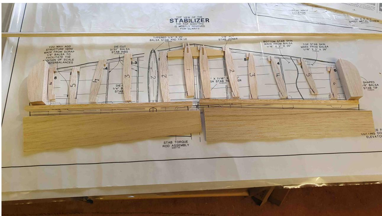
And here's the almost complete tailplane with elevators dry hinged in position. Note the cut out for the balance tab which is still to be fitted to the elevators.
