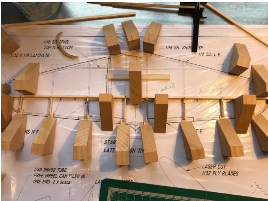
Gluing it all together almost defeated my steel and magnetic building board. There just isn't room between the parts to retain the spars; prop all of the edges; fit each rib centrally on the spar and leading/trailing edges.
