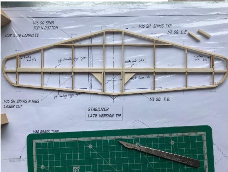
Major lesson - draw the intended changes on the plan before building the piece. That way all of the figuring out and interdependent gluing challenges would at least have been thought about in advance. I would probably have put the elevator in the right place too.
