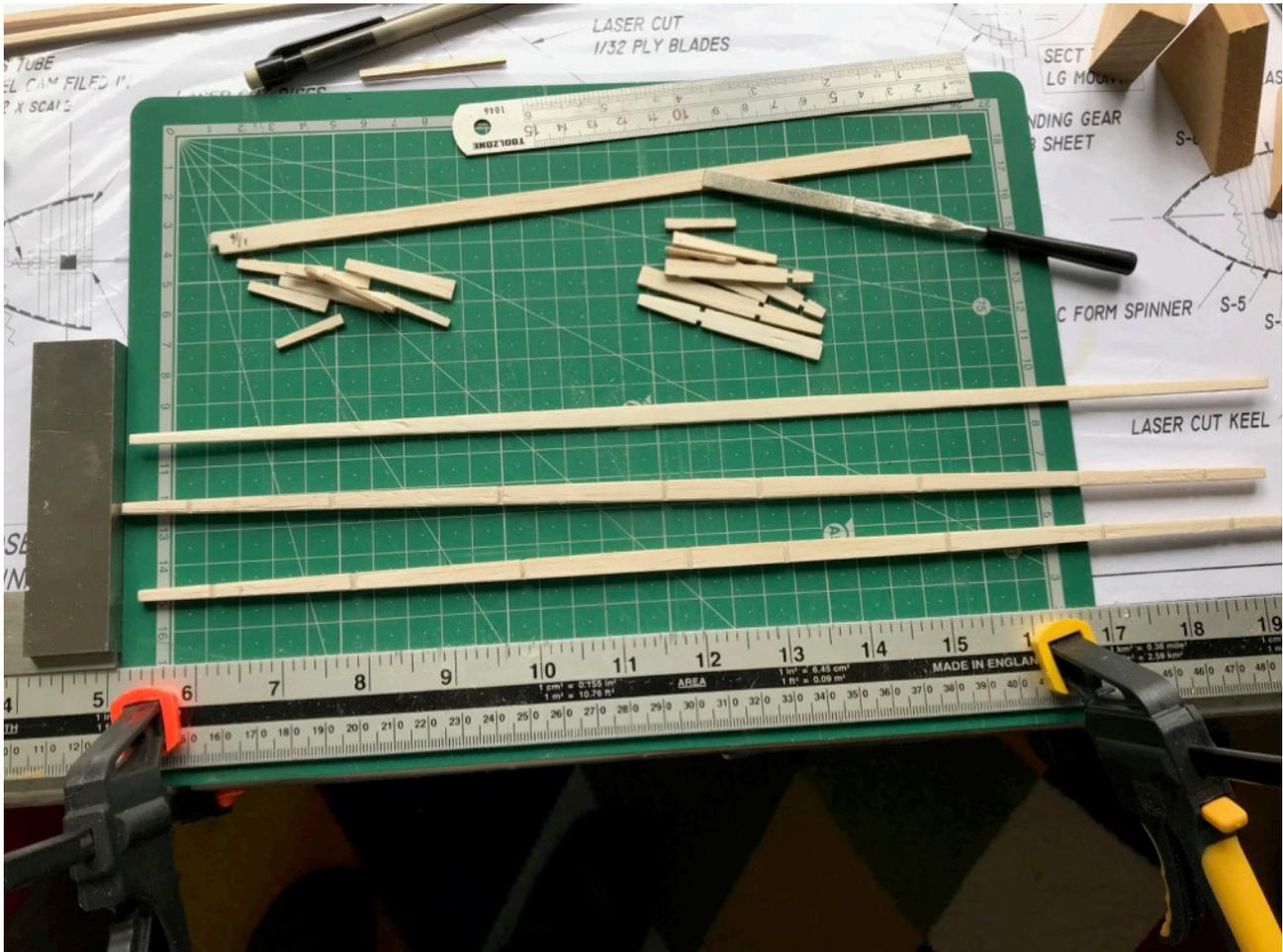
spar, aided flat and level 1/16" slots. It still left me with a tiny bit of each rib to loose, but at least sanding to fit is a familiar operation.
