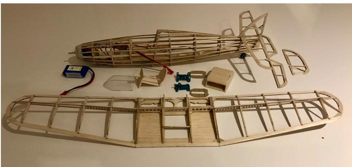
I took a punt on finished weight and have overpowered it possibly with a 10g brushless motor and 2S battery. On the other hand the finished all up weight of 77g compares very well with a similar sized eFlite UMX SBach. Yet to fly, yet to find out! Incidentally, finished for free flight the auw is likely sub 30g.
