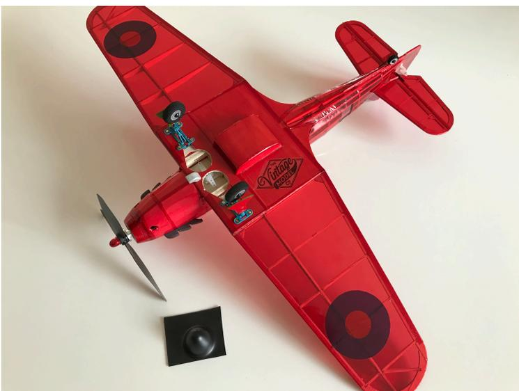
The model is covered with Solite transparent red instead of the very nice tissue supplied, with the paper/covering process extended to behind the cockpit to imitate the standard Hurricane metal sheeting look. Insignia were downloaded from The Vintage Model Company and printed onto decal paper from MrDecalPaper.
