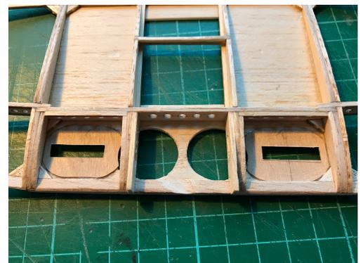
More rugged stuff was added to the wing centre section for the retracts - a 1mm balsa plate; 1mm ply forward plate and 0.4mm ply leg reinforcement internally; along with 2 rib reinforcements and 2 additional riblets to enable the retract mechanism to clear the covering. Not a lot of weight (10g with fittings and servo), but the worst impact is likely to be from the resulting change to the centre section aerofoil.
